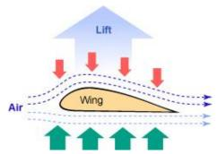
The pressure exerted down by fast moving air (red arrows) is less than the pressure exerted up by slow moving air (green arrows).
